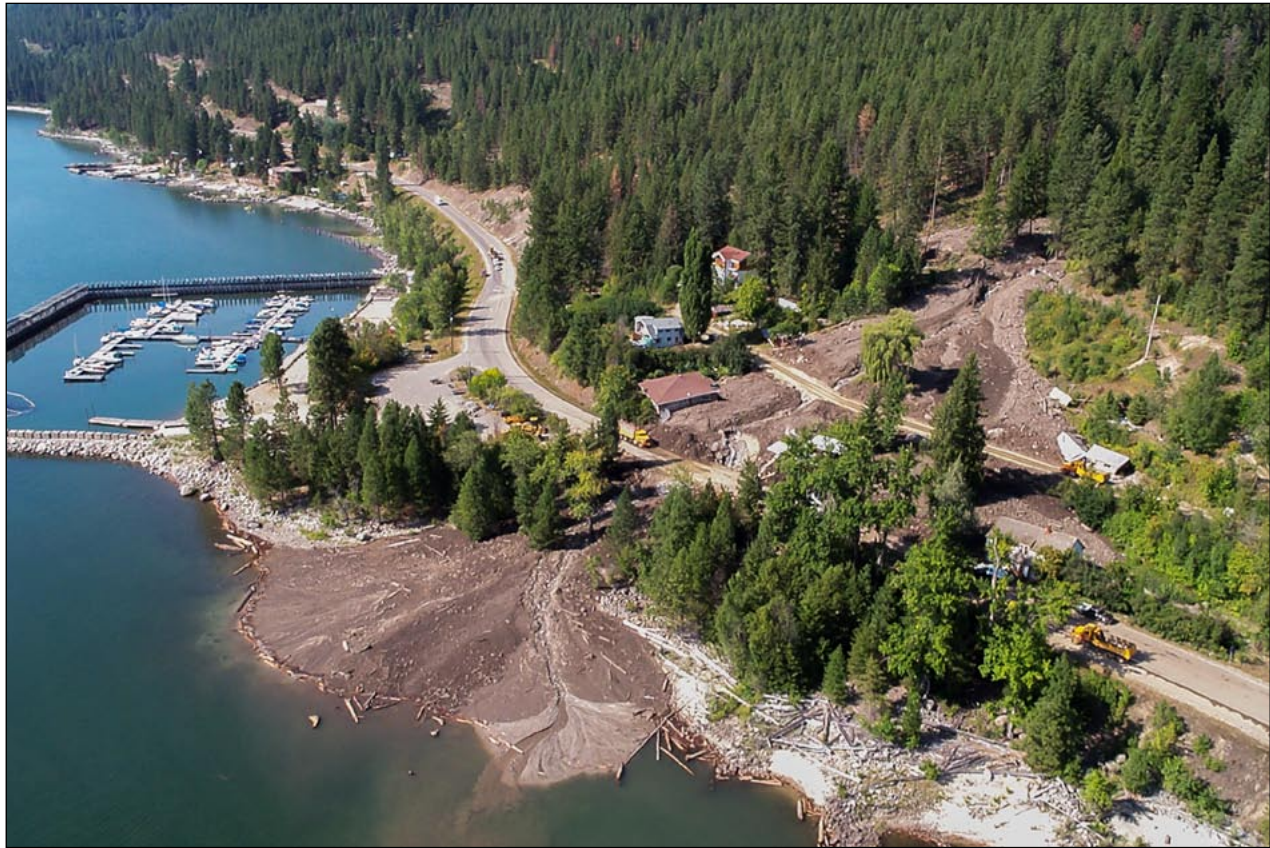
FIGURE 1 Deposition zone of a debris flow that originated from the 2003 Kuskanook Fire, north of Creston, B.C. The fire burned in 2003, and the debris flow occurred in August 2004 during a high-intensity rainstorm. (Photo: P. Jordan)
