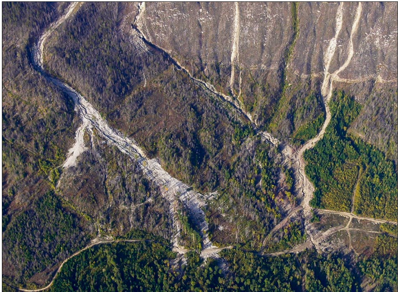
FIGURE 9 Debris flows originating in the area burned by the 2003 Ingersoll Fire near Burton (Arrow Lakes) after a long-duration, frontal rainstorm in October 2005. (Photo: P. Jordan)
